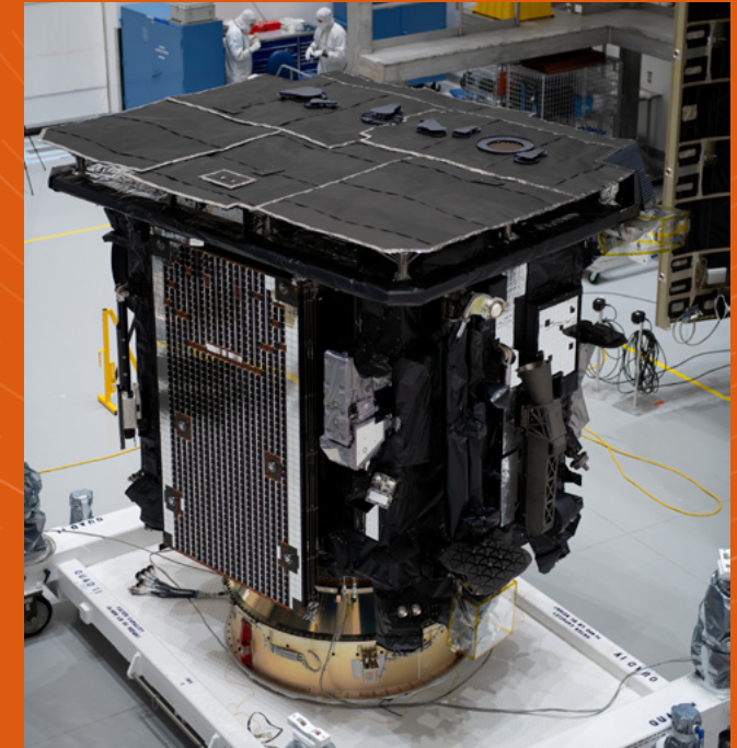
Figure 8: The Solar Orbiter spacecraft before launch, clearly showing the black heat shield on top. The heat shield was coated by Irish company Enbio. © ESA, S Corvaja.
