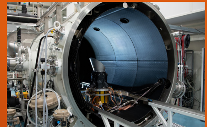
Figure 9: A PLATO camera mounted inside the VTC-1.5 Space Simulator for testing, using liquid nitrogen to keep it around -80 °C. © ESA, Matteo Apolloni.
