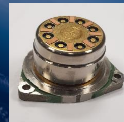
CVG2 Gyro Sensing Element
