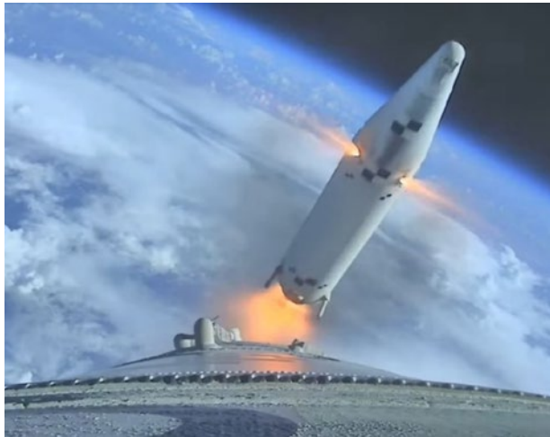
Figure 8: Ariane 6 rocket booster separation, captured by Réaltra's cameras onboard the launcher's maiden flight from Europe's Spaceport, Kourou, French Guiana © ESA/ ArianeSpace/Réaltra Space Systems Engineering
