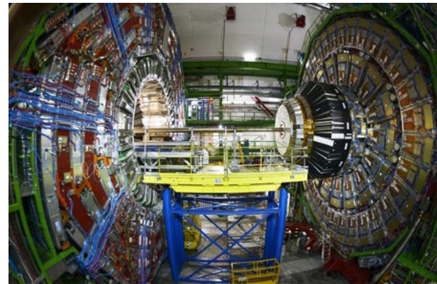
Figure 39: Compact Muon Solenoid (CMS) detector; one of two large general-purpose particle physics detectors built on the Large Hadron Collider (LHC) at CERN © Maximilien Brice, CERN
