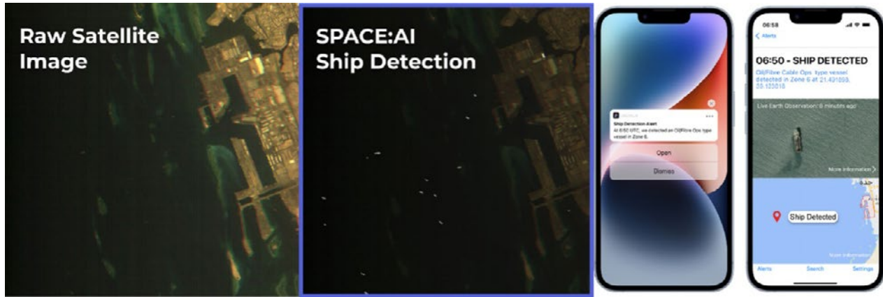
Figure 24: SPACE:AI detects and classifies all vessels near a port in 90 seconds, instantly relaying intelligence to users for real-time interaction © Ubotica
