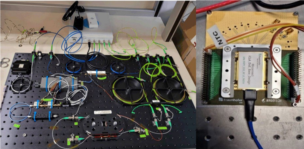
Figure 59: Benchtop setup and integrated circuit to demonstrate the use of photonic technology for generating low phase noise RF signals © DCU
